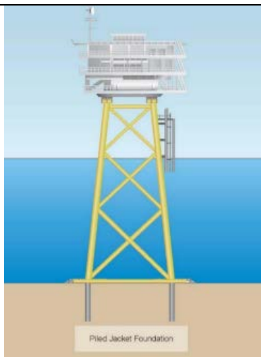
Figure 11 Sub-station on fixed jacket substructure
